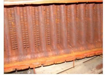
Boiler 1 and 2 were then disassembled, and four sections from each unit were sandblasted for a clearer look at the cast iron surface. All sections showed nearly identical levels of wear, which proved inconsequential. When compared side-by-side with a new heat exchanger, it was hard to see any significant differences in the surface between the new and returned sections.
